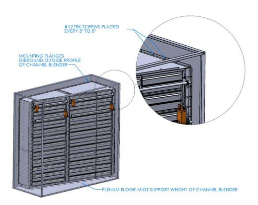
The installation method of the Channel Blender to an AHU OEMs mixing box can vary from OEM to OEM based size & weight of the Channel Blender and on the OEMs panel design.
