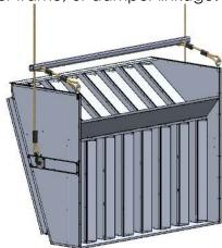
Channel Blenders with horizontal blades for side entry mixing boxes are designed to sit on the floor of the AHU. There is a base that includes fork lift pockets to lift and move the unit.
